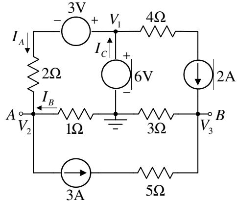
$$\left. \begin{aligned} V_1 &= 6V \\ -\frac{1}{2}V_1 + \frac{3}{2}V_2 &= -\frac{9}{2} \Rightarrow V_2 = \frac{1}{3}V_1 - 3 \\ \frac{1}{3}V_3 &= 5 \end{aligned} \right\} \Rightarrow \boxed{V_1 = 6V}, \quad \boxed{V_3 = 15V}, \quad \boxed{V_2 = -1V}$$
