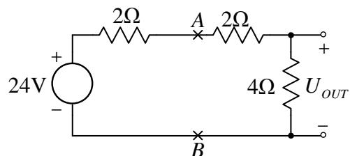
$$U_{OUT} = \frac{4\Omega}{4\Omega + (2\Omega + 2\Omega)} \cdot 24V \Rightarrow \boxed{U_{OUT} = 12V}$$
