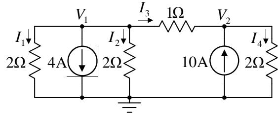
$$\left. \begin{array}{l} 2V_1 - V_2 = -4 \\ -V_1 + \frac{3}{2}V_2 = 10 / \cdot 2 \end{array} \right\} \Rightarrow \left. \begin{array}{l} 2V_1 - V_2 = -4 \\ -2V_1 + 3V_2 = 20 \end{array} \right\} + \Rightarrow 2V_2 = 16 \Rightarrow \boxed{V_2 = 8V}, \boxed{V_1 = 2V}$$
