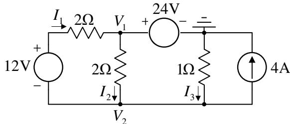
$$\left. \begin{aligned} V_1 &= 24\text{V} \\ -\left(\frac{1}{2\Omega} + \frac{1}{2\Omega+0}\right)V_1 + \left(\frac{1}{2\Omega+0} + \frac{1}{2\Omega} + \frac{1}{1\Omega} + 0\right)V_2 &= -4\text{A} - \frac{12\text{V}}{2\Omega} \end{aligned} \right\} \Rightarrow \left. \begin{aligned} V_1 &= 24\text{V} \\ -V_1 + 2V_2 &= -10 \end{aligned} \right\}$$
