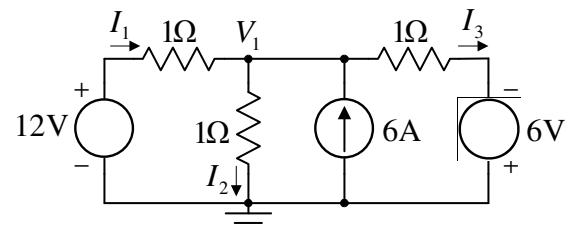
$$I_1 = \frac{12V - V_1}{1\Omega} \Rightarrow I_1 = 8A, \quad I_2 = \frac{V_1 - 0}{1\Omega} \Rightarrow I_2 = 4A,$$
