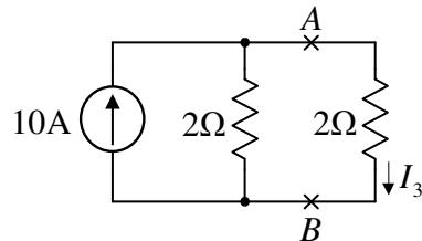
$$I_3 = \frac{2\Omega}{2\Omega + 2\Omega} \cdot 10A \quad \Rightarrow \quad I_3 = 5A$$
