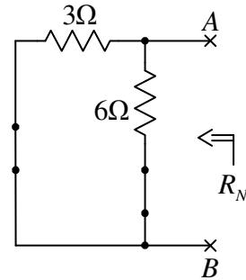
$$\text{Kontura } K_1: \quad I_1 \cdot 6\Omega - 12V = 0 \quad \Rightarrow \quad I_1 = 2A \quad R_N = 6\Omega \parallel 3\Omega = 2\Omega$$
