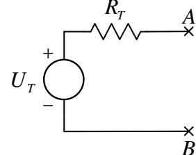
$$U_T = U_{OV} = \frac{6\Omega}{6\Omega + 3\Omega} \cdot 36V = 24V$$
