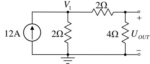
$$\text{MPČ: } \left( \frac{1}{2\Omega} + \frac{1}{6\Omega} \right) V_1 = 12A \Rightarrow V_1 = 18V$$
