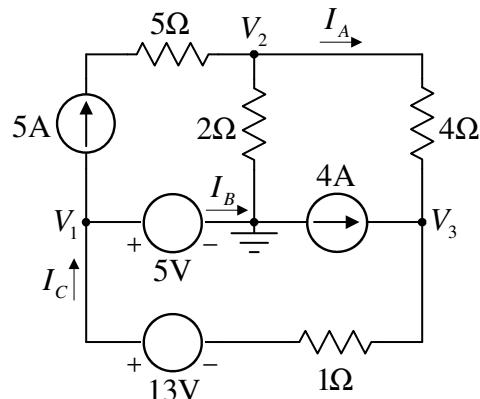
$$\left. \begin{array}{l} V_1 = 5V \\ \frac{3}{4}V_2 - \frac{1}{4}V_3 = 5 \Rightarrow V_3 = 3V_2 - 20 \\ -V_1 - \frac{1}{4}V_2 + \frac{5}{4}V_3 = -9 \end{array} \right\}$$
